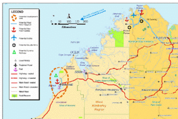
Figure 42 Infrastructure requirement for bauxite mine at Mitchell Plateau, alumina refinery in vicinity of Broome Source: Developing the West Kimberley's Resources 2005 Page 130
